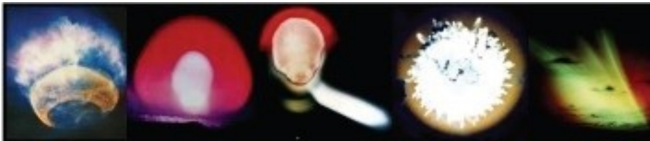
Figure 4. From left to right, the ORANGE, TEAK, KINGFISH, CHECKMATE, and STARFISH high-altitude nuclear tests conducted in 1958 and 1962 by the United States near Johnston Island in the mid-Pacific. Burst conditions for each were unique, and each produced strikingly different phenomena and different enhancements of the radiation belts. 18
